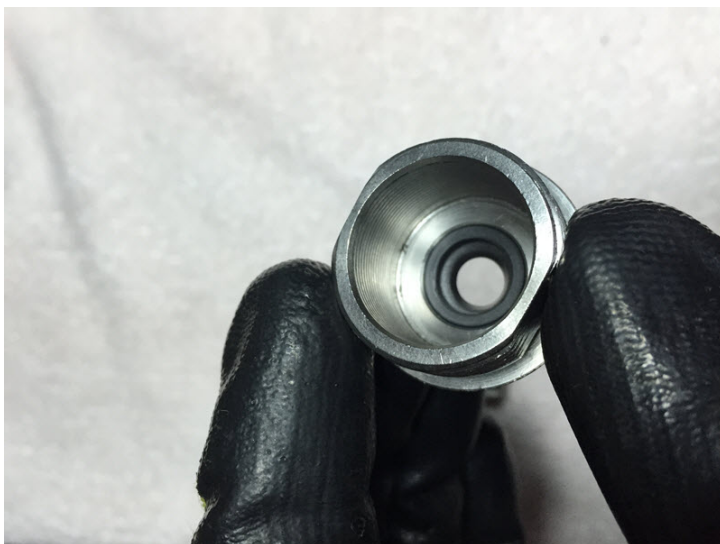
Install seal in housing. Make sure the o-ring is properly seated in seal. Seal should not spin freely in housing.
