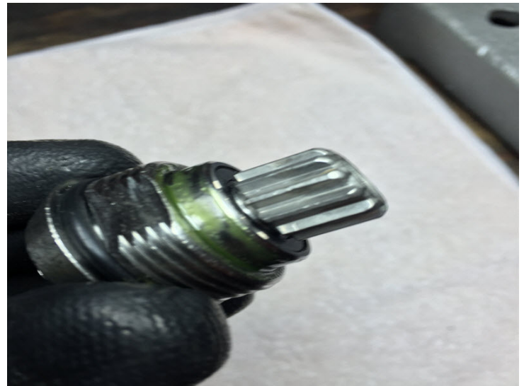
Apply an even coat of Loctite to second bearing before pressing into housing.
