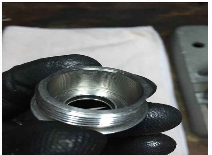
Remove all Loctite adhesive from inside of housing. Note: Bearings must insert and remove freely.
