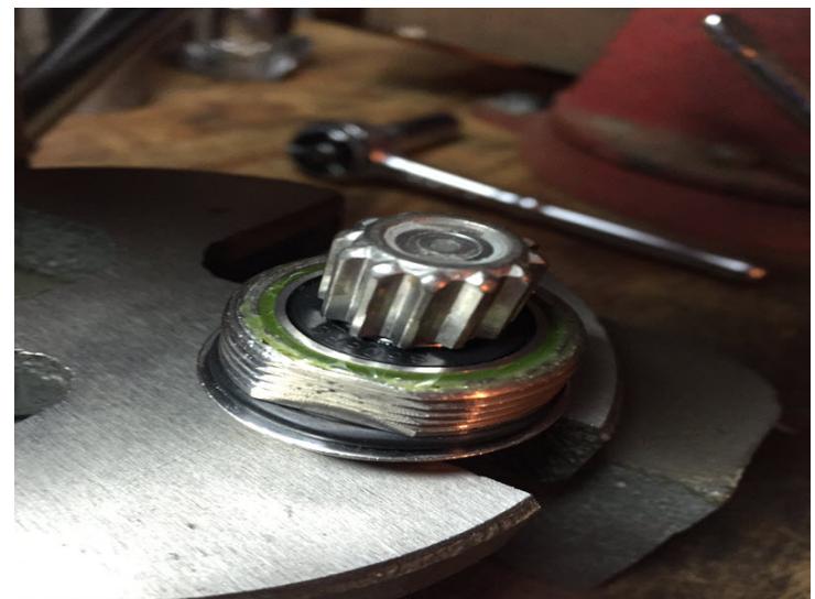
Shows bearings fully pressed into housing.
