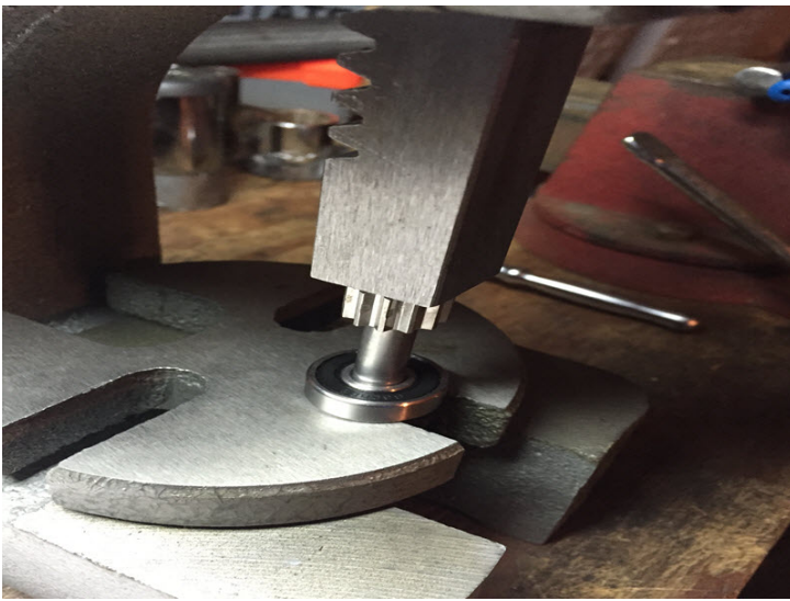
Press first bearing down to the drive gear. (for Advance blade assembly see diagram)
