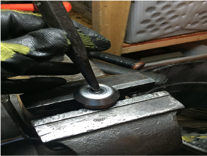
Using a center punch, remove shaft from housing. Be careful not to damage housing assembly or shaft.
