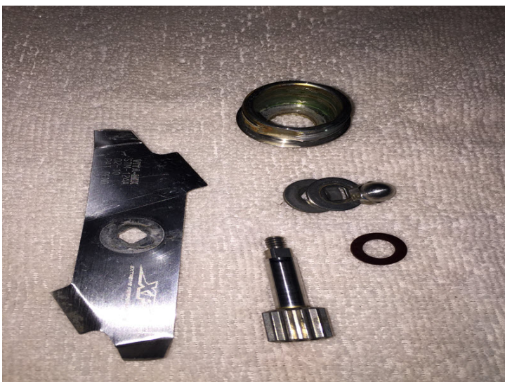
Thoroughly clean blade assembly components.
