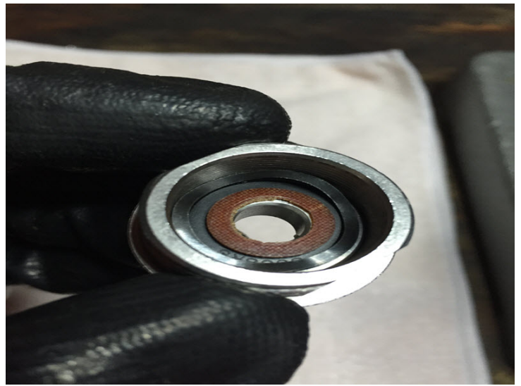
Insert second bearing wave spring and spacer into housing. (keep's everything aligned during pressing)
