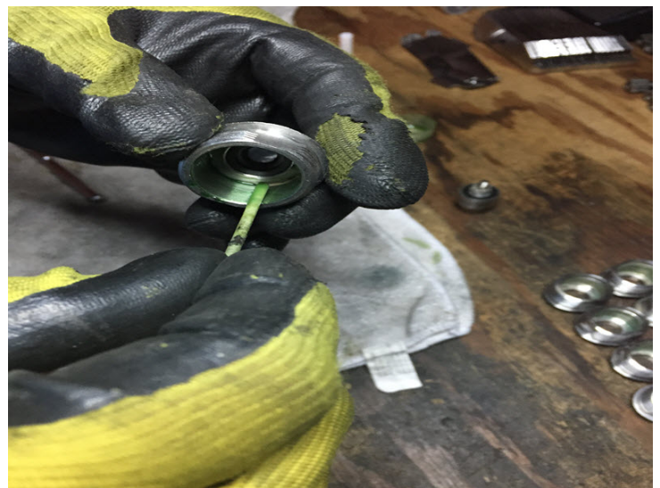
Spread Loctite evenly inside the housing. A tooth-pick or cut off Q-Tip works fine for this.
