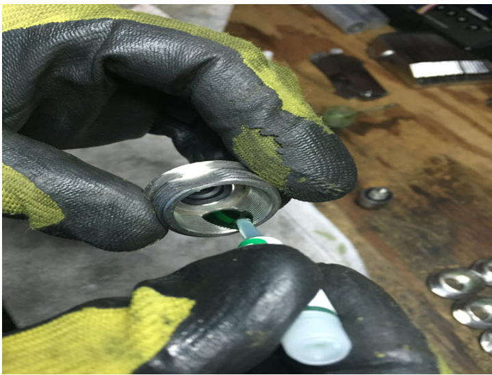
Apply Loctite to inside of housing. Only requires a drop about 3/8 of an inch in size.
