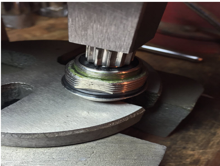
Press bearing assembly into housing slowly to prevent damage to the seal.
