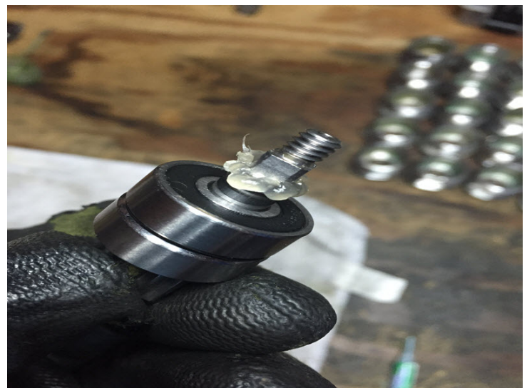
Apply grease around edge of shaft. This helps prevent damage to seal when pressing bearings into housing.
