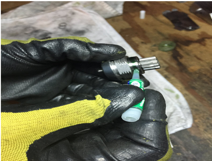
Partially insert bearing assembly into housing to allow for Loctite to be applied to the second bearing.
