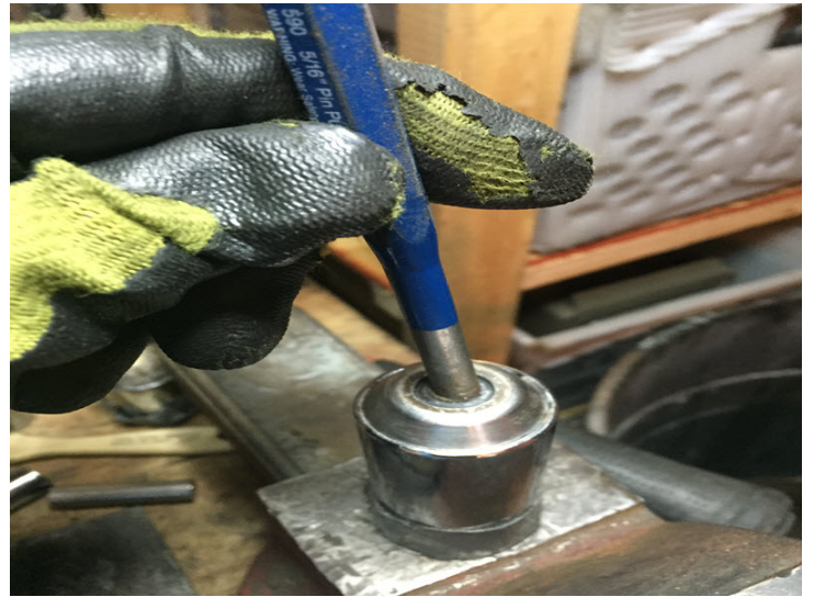
Finish removing bearings with a large punch. Using a 27mm 12 point socket will prevent damage to housing.
