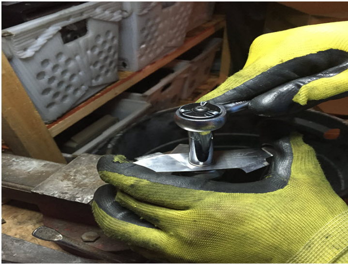
Remove blade from housing assembly.
