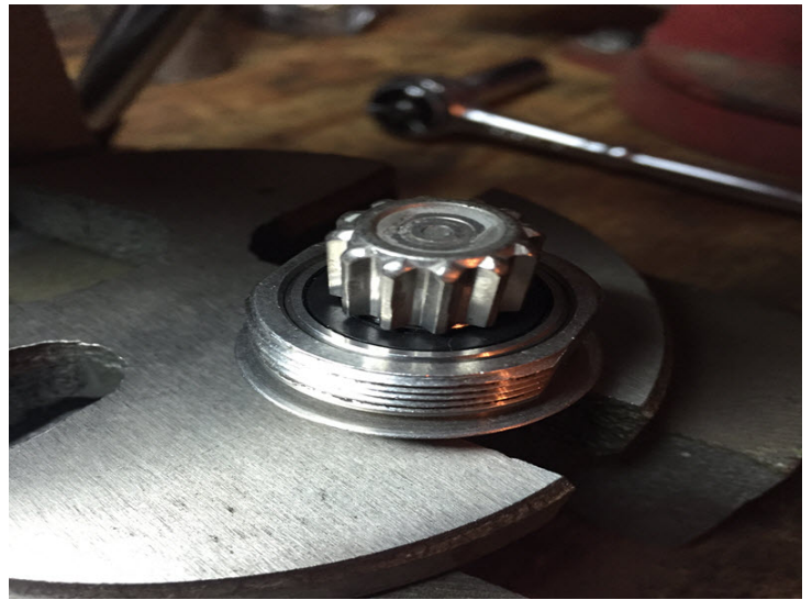
Shows the bearings pressed all the way into the housing assembly.
