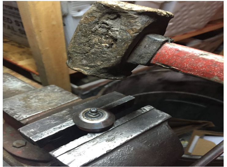
Place housing on vise and carefully remove shaft with a brass mallet.
